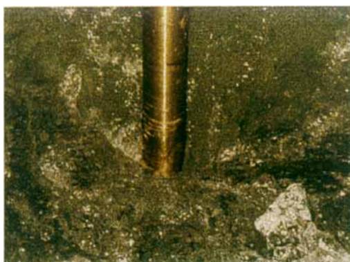
Vortex around impeller shaft
